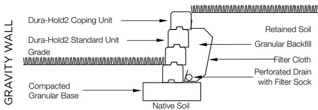
Cross sections are examples, and must not be used for construction.
