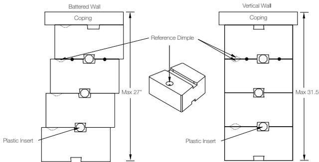
All cross sections are examples, and must not be used for construction.
